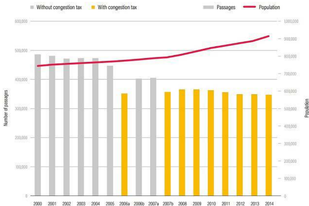
Figure 21: Traffic volume in Stockholm declined and has remained below pre-congestion-charge averages even as population increases. 2006b and 2007a mark the time between the end of the trial period (July 2006) and beginning of the official implementation of charging scheme (August 2007)
