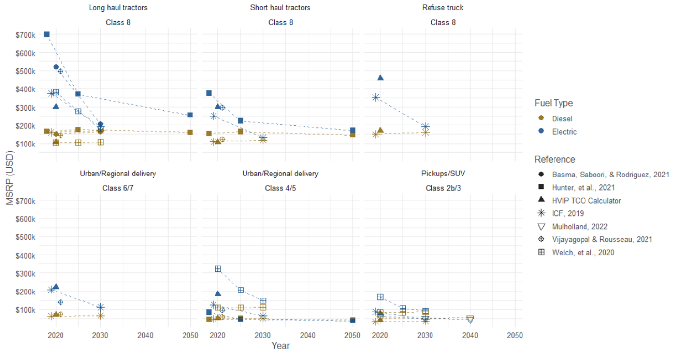
Figure I-1. Projected current and future MSRP ($) for BETs and baseline trucks with sources
